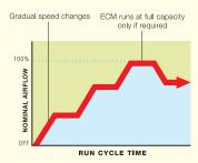
Extended run times at reduced speeds help to control humidity and reduce noise.
